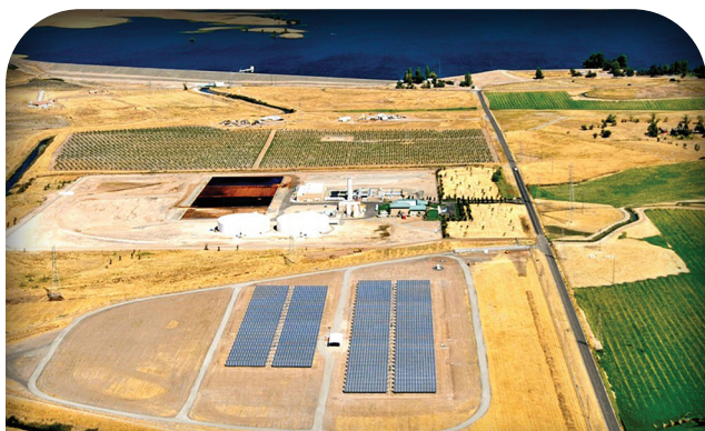
Figure 1. Two silicon-based tracking arrays (PV1) were installed in 2008, followed by 2009 deployment of a thin-film array (PV2) in the vacant lot at left. (Credit: SSJID)
