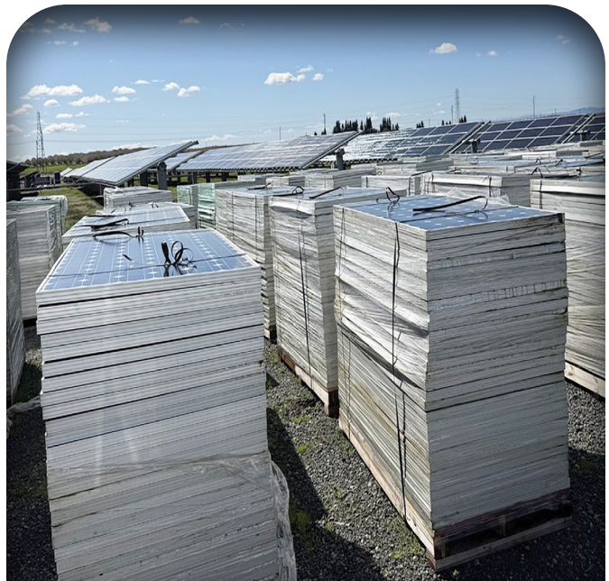
Figure 8. Legacy c-Si modules were stockpiled for transport and processing by an out-of-state recycling services provider. (Credit: SSJID)
